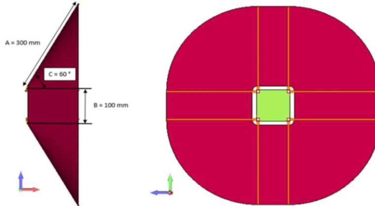
Figure 6: Geometry of the F-TPS truncated cone
