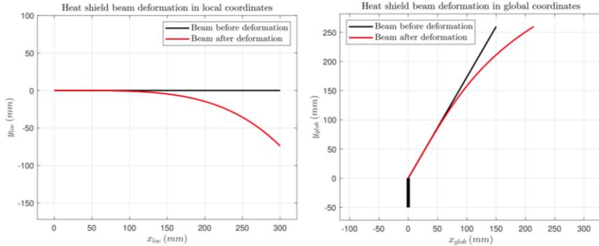
Figure 8: F-TPS Nitinol beams maximum deformation in local and global coordinates
