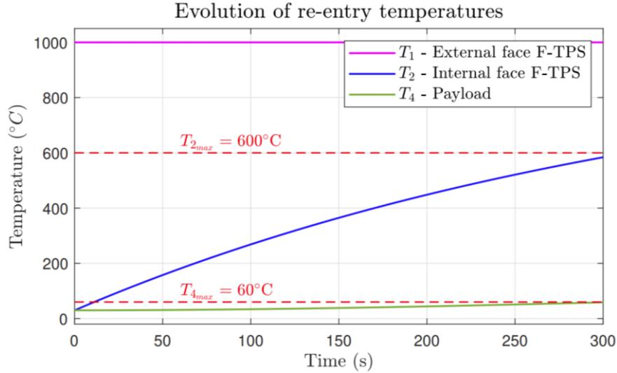
Figure 7: Temperatures for conductive F-TPS and MLI
