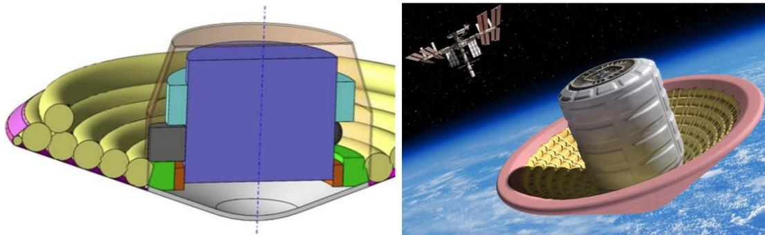
Figure 1: EFESTO's concept design & NASA's HIAD
