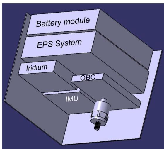
Figure 5: Physical check of clearance in 1U payload module
