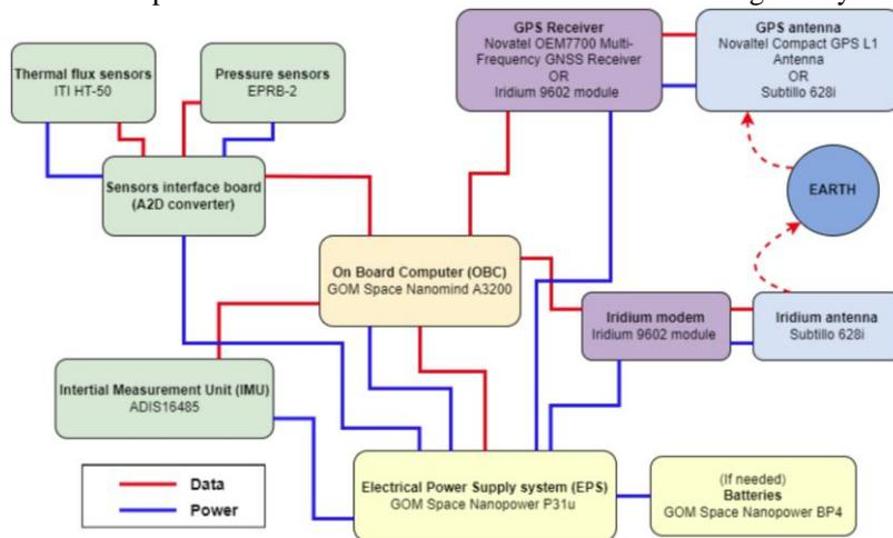
Figure 4: Payload module block diagram
