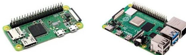
Figure 19: ASTREOS 1 Raspberry Pi4 and Pi0
