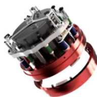
Figure 20: ASTREOS 1 Separation and recovery device
