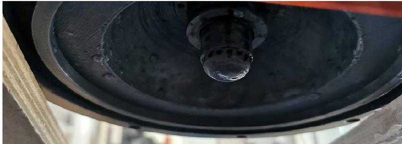
Figure 29: Additive manufacturing mock-up of the pintle injector
