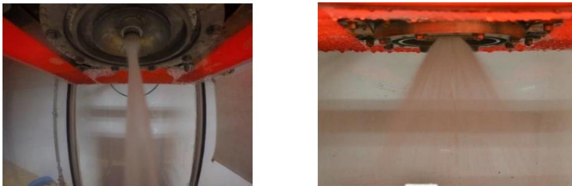
Figure 22: Ethanol circuit flow and Ethanol + LOX circuits together
