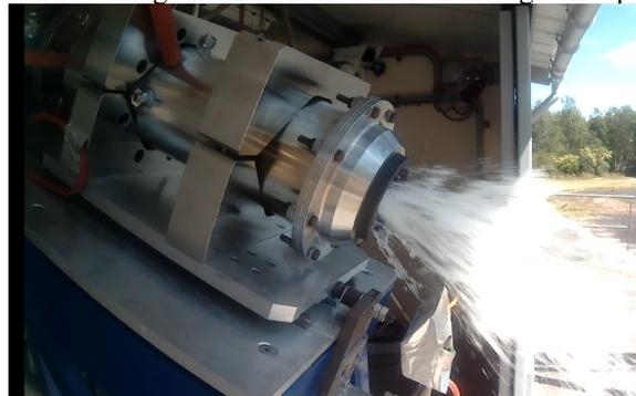
Figure 16: Ethanol circuit flow check
