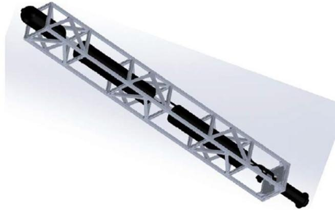
Figure 18: “Battleship” structure for stage tests
