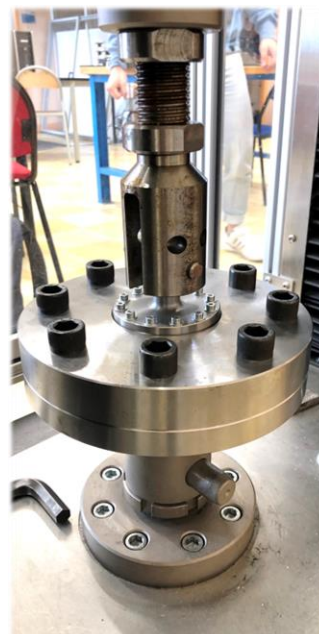
FIGURE 11 – Out-of-plane pull-out test result on the composite baseplate
