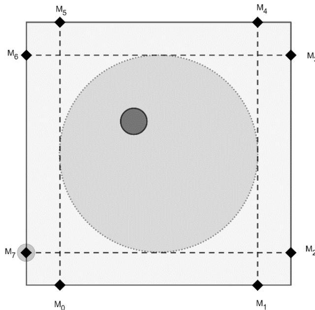
Figure 3: 2D representation of the Smartcatcher capture zone. The landing area is the light grey disk; the rocket is the dark grey disk; the mobile cables correspond to the dotted lines; each cable is controlled by 2 stepper motors, respectively M0 - M5, M1 - M4, M2 - M7 and M3 - M6
