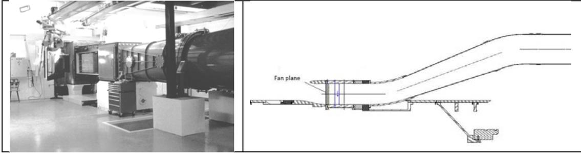
Figure 12: S3Ch wind-tunnel (left) and model set-up with suction circuit (right).
