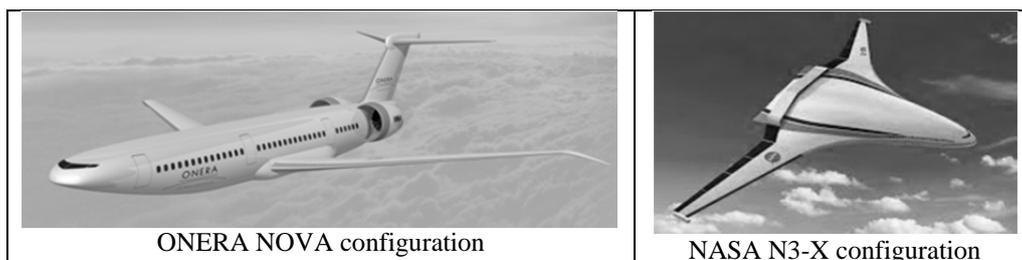
Figure 1: Aircraft innovative configurations with BLI engine installations.
