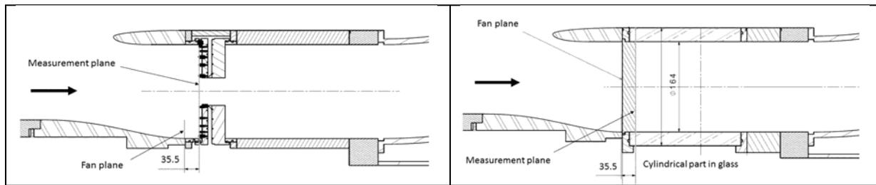
Figure 13: Model for total pressure (left) and PIV (right) measurements.
