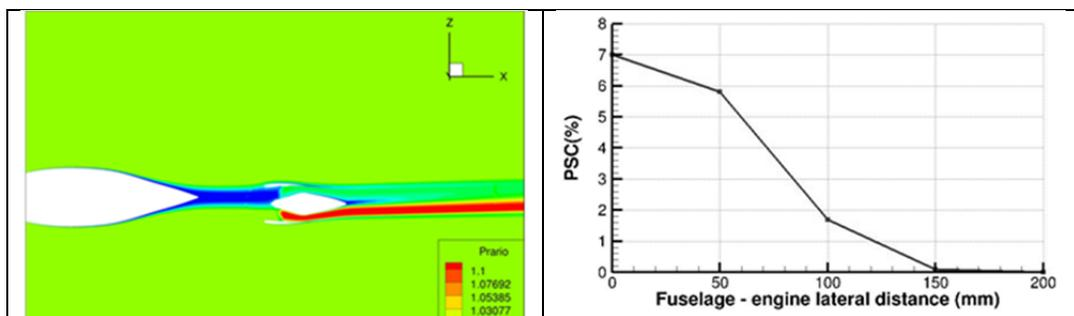
Figure 6: Total pressure around generic configuration at cruise Mach number 0.82 (left) and benefit on engine power according to the lateral position of the engine (right).
