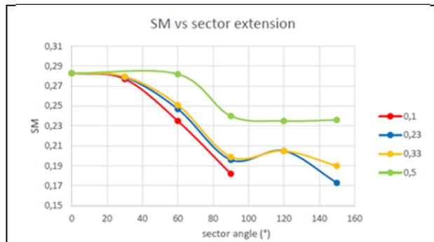
Figure 9: Surge margin versus the wireframe sector angle for the different porosities.
