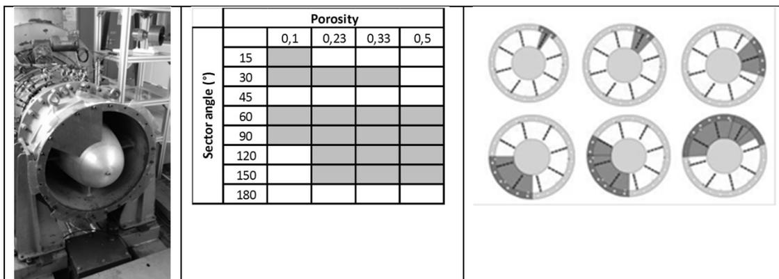
Figure 7: CME2 bench with wireframe (left), wireframe sector angles and porosities (middle and right).
