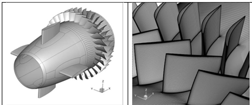
Figure 10: CME2 configuration and detailed view of the mesh (the shroud is blanked in these views).
