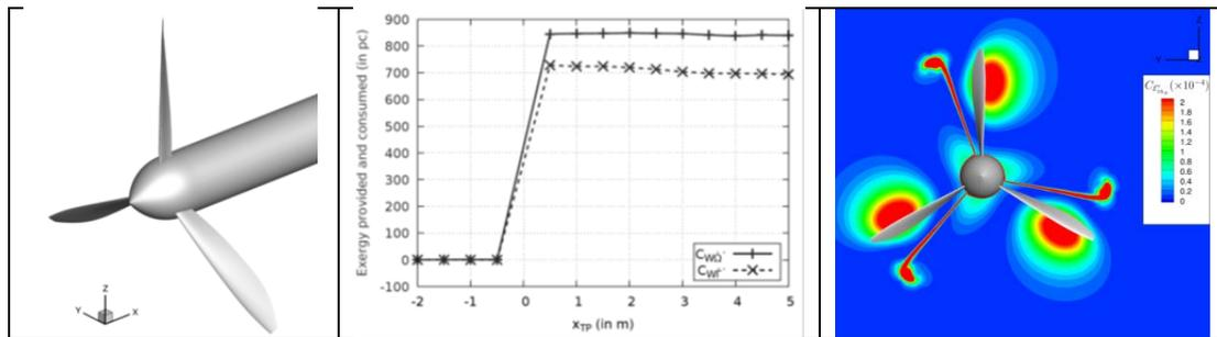
Figure 3: HAD-1 propeller (left), exergy provided and consumed by the system (middle), contours of thermocompressible exergy at propeller level (right) [15]
