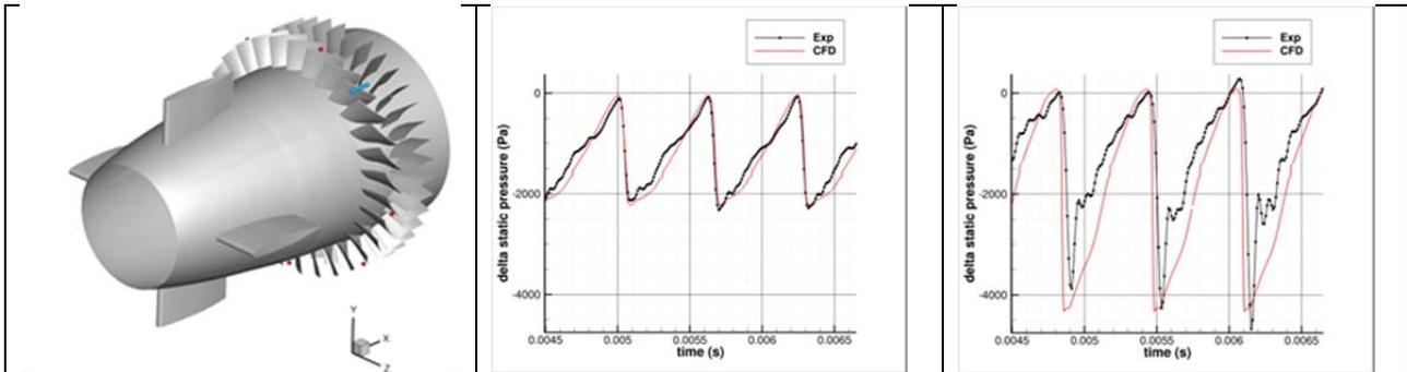
Figure 11: Probes location (left) and comparison of experimental and numerical pressure signals without distortion grid (middle) and with a 60° and 33% porosity grid (right) (pressure probe at shroud near rotor leading edge).
