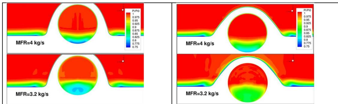
Figure 17: Total pressure in fan plane for different inlet massflows for inlet 1 (left) and 2 (right) - Mach 0.82 Sideslip angle 0°.
