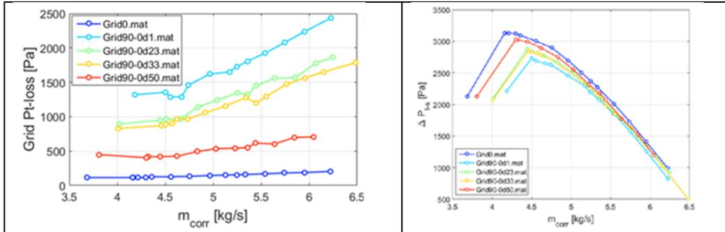
Figure 8: Total pressure loss due to 90° wireframe for porosities 0, 0.1, 0.23, 0.33, 0.50 (left) and fan pressure drop versus corrected massflow (right).
