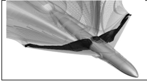
Figure 2: Volumes of integration for the viscous (grey) and wave (black) components of exergy for the NASA-CRM configuration at cruise [13]
