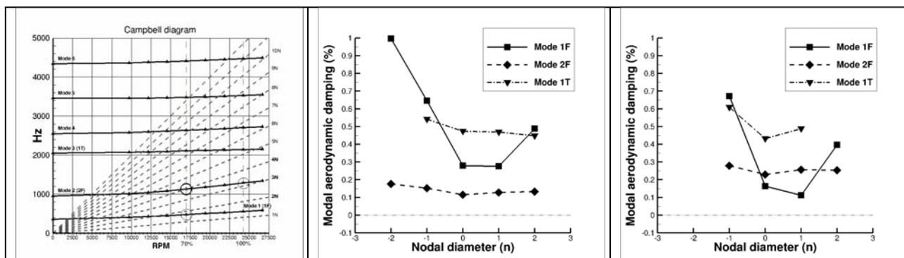
Figure 19: Campbell diagram for the first six modes of the blade (left) and aerodynamic damping for the first three modes: **without distortion** (middle), **with distortion** (right).
