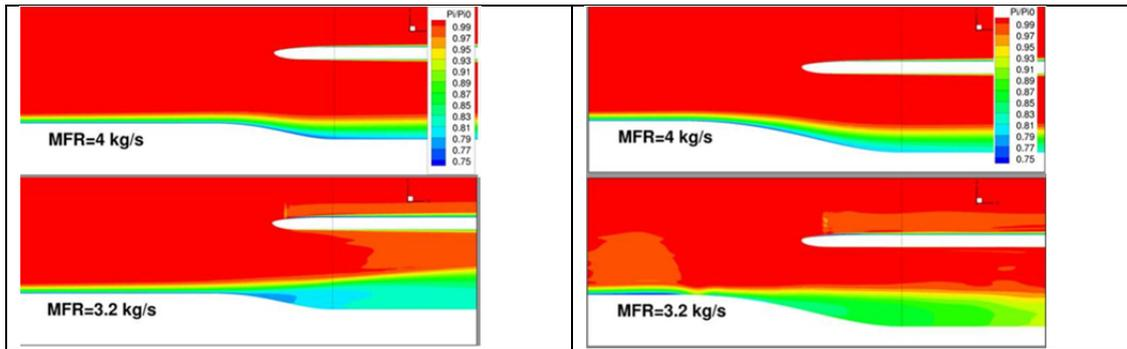
Figure 16: Total pressure in symmetry plane for different inlet massflows for inlet 1 (left) and 2 (right) - Mach 0.82 Sideslip angle 0°.
