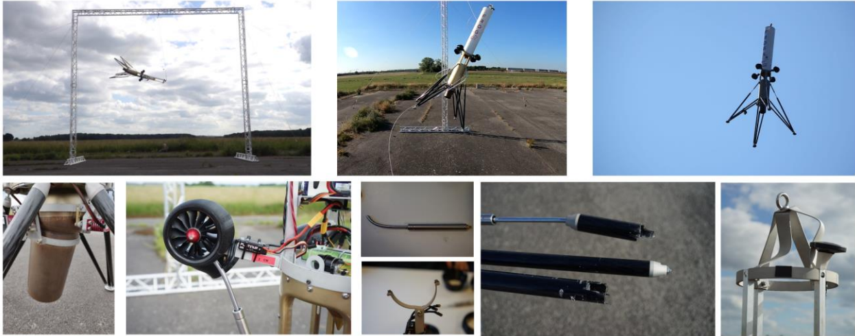
Figure 5: Various RUD (Rapid Unscheduled Disassembly) of FROG-T during tethered flights
