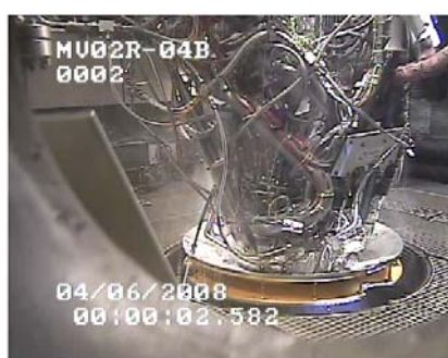
Fig. 3 – View of firing engine in test cell
