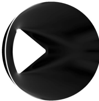
Figure 2 Numerical schlieren of the wake flow over the Apollo reentry capsule
