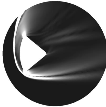
Figure 6 Numerical schlieren of the wake flow over the Apollo reentry capsule
