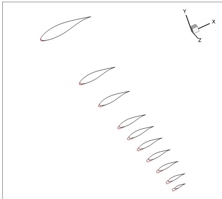
Figure 2: Ice formation on the blade elements of the AEOLOS 30 kW wind turbine
