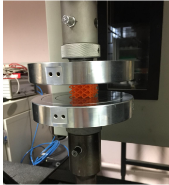
Figure 4: Polymeric samples: compression tests
