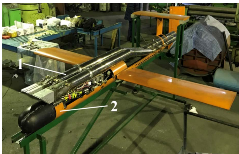
Figure 8: Assembly of the UAV with two paired PDE-based TMs: 1 – TM, 2 – UAV
