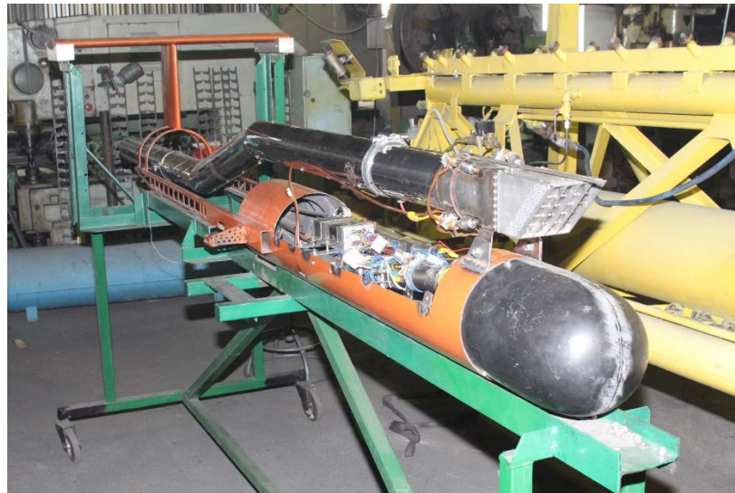
Figure 6: Assembly of the UAV with the PDE-based TM: general view
