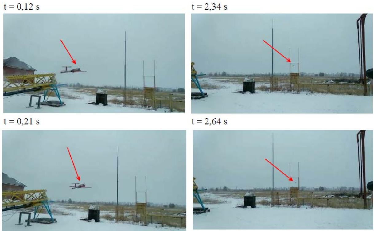
Figure 10: Video frames of the UAV powered with one TM in the flight. Arrows shows the position of the UAV. Time is counted from the instant of UAV separation from the catapult.
