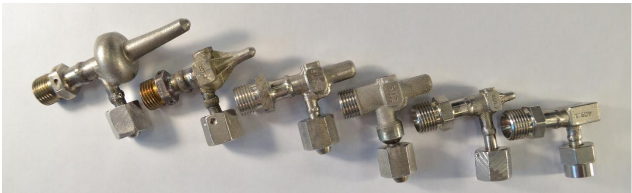
Fig. 7: Manufactured igniters (from left to right): d=3.8 mm, d=2.4 mm, d=1.8 mm, d=1.8 mm CoCr, d=1.3 mm, d=0.9 mm.
