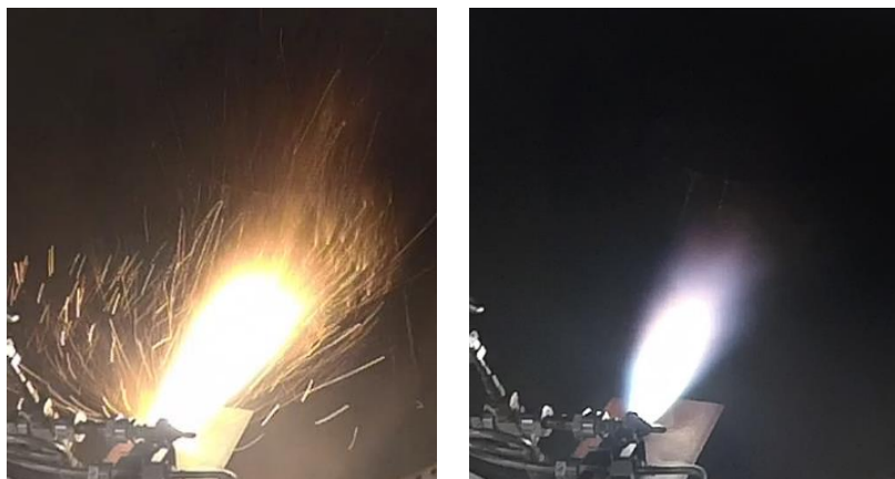
Figure 16: Ablation of metal just after ignition (left) and subsequent normal igniter operation (right)
