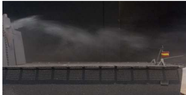
Figure 8: Flow visualization using smoke.
