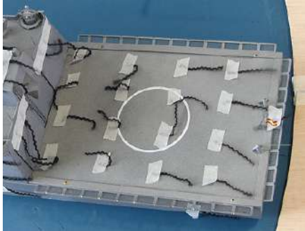
Figure 7: Flow visualization using wool plumes.
