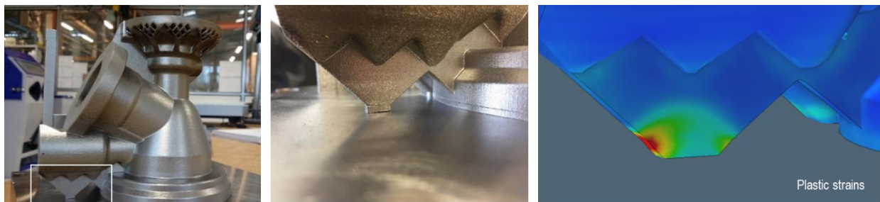
Figure 22: Cracking of a valve casing due to high residual stresses predicted by Simufact
