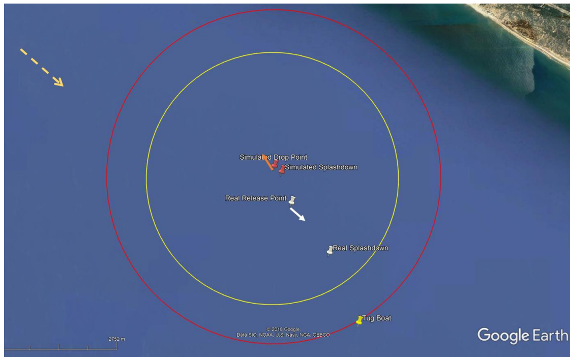
Figure 9 - FLPP LPSR Drop Test: Foreseen vs Real Drop and Impact Points
