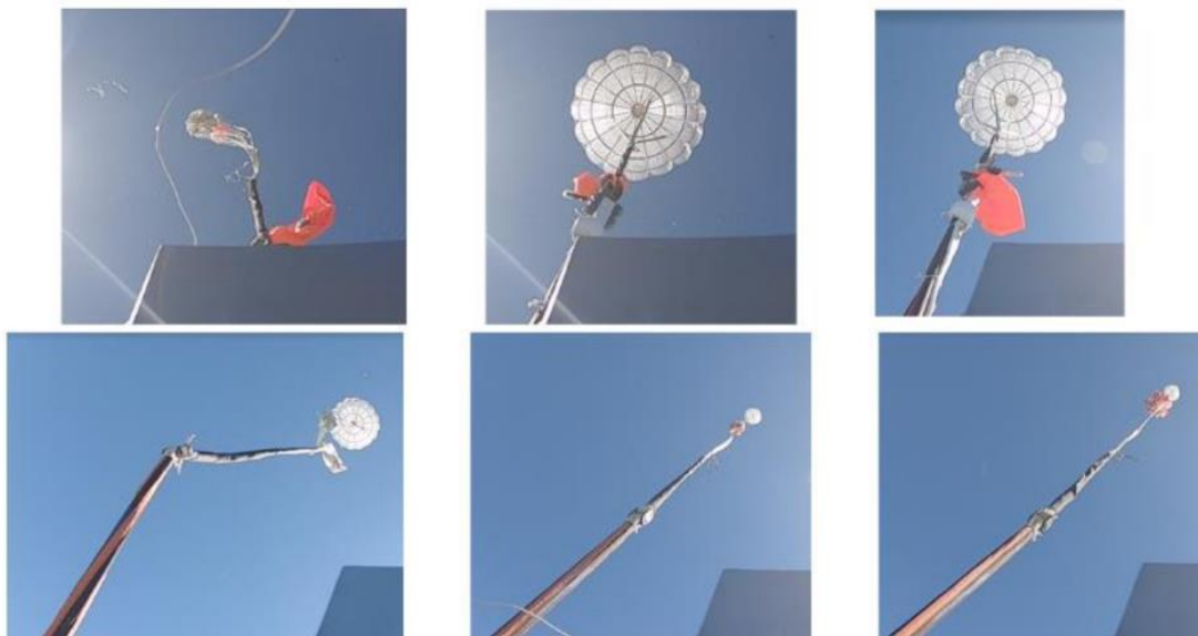
Figure 7 - FLPP LPSR Drop Test: Drogue Stage (inflation up-row, cutting & pulling main bottom-row)
