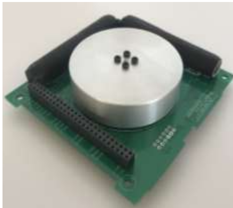
Figure 3: Image of the ADCS board with the actuators: wheel and magnetorquers (courtesy of Theia Space).
