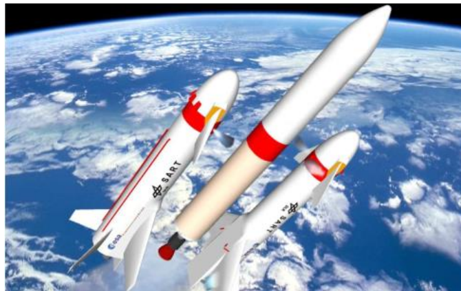
Figure 1: Artist's impression of the Liquid Fly-Back Boosters disconnecting from the center core
