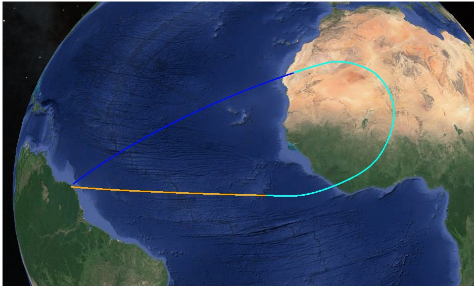
Figure 37: Illustration of return to launch site with a propelled air-breathing phase using SABRE engines. Orange trajectory corresponds to the ascent phase, then cyan trajectory is the ballistic phase, the re-entry and u-turn of the first stage while the blue trajectory corresponds to the air-breathing propelled phase to return to the launch site.
