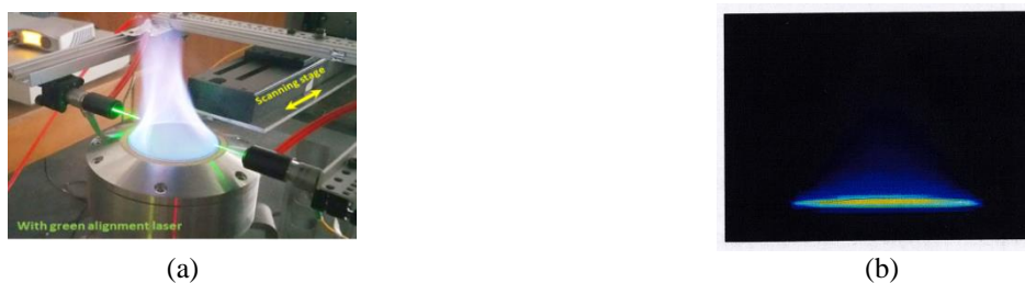
Figure 5: Image of (a) burner McKenna and (b) of a configuration of stable flat flame for flows of 20\text{ mL/s} of air and 2\text{ mL/s} of methane
