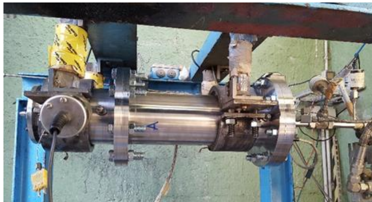
Figure 4: 1000 N breadboard integrated on the test bench
