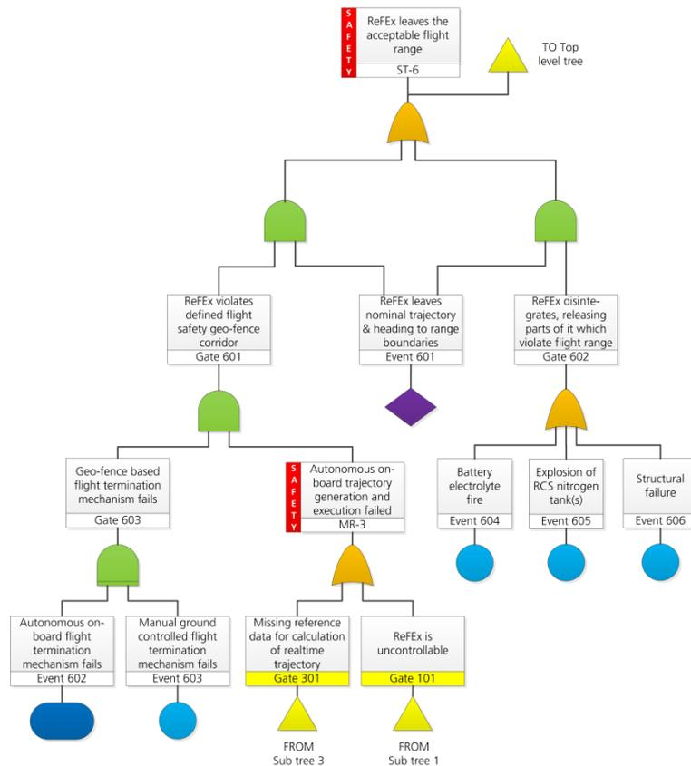
Figure 8: Sub-tree 6 - *ReFEx leaves the acceptable flight range*
