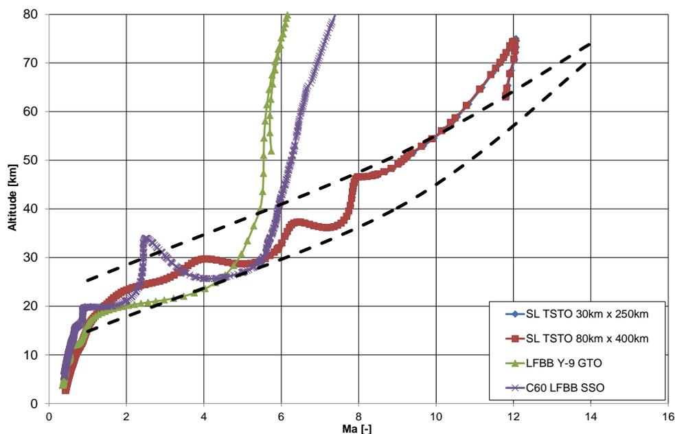
Figure 1: Re-entry trajectories and related RLV (Reusable Launch Vehicle) corridor for different winged RLV first stages including the SpaceLiner (SL), the Liquid Fly Back Booster (full-scaled final version LFBB Y-9, sub-scaled micro methane LFBB C60)
