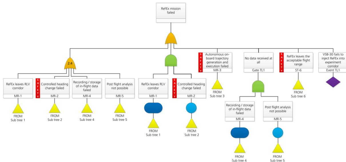
Figure 6: ReFEx top-level fault tree
