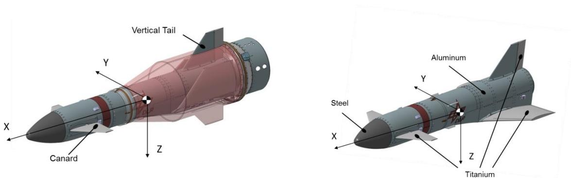
Figure 3: Detailed view of ReFEx in stowed/launch configuration (left) & re-entry configuration (right) [10]
