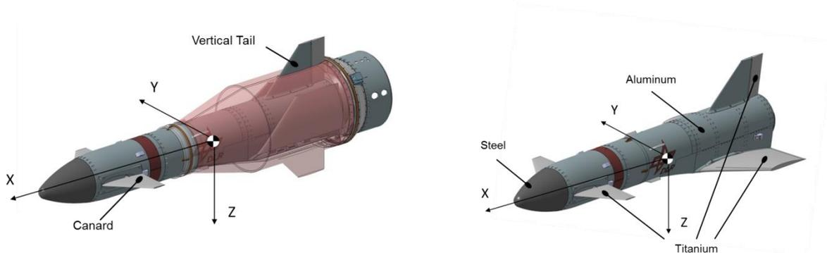
Figure 3. ReFEx is stowed underneath a triple shell fairing with the wings folded. The antennas for GPS (wrap-around) and telecommunication are all located outside of the fairing. This allows the fairing to be fabricated of carbon fibre, which is opaque to RF transmissions, saving mass and improving rigidity over a glass-fibre variant.
