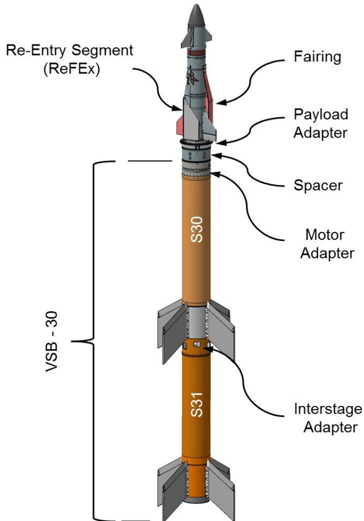
Figure 2: ReFEx in its launch configuration atop the VSB – 30 (one fairing half omitted for illustration purposes) [10]
