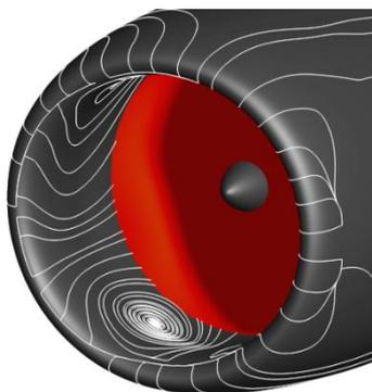
Figure 4: Streamlines near inlet surface
