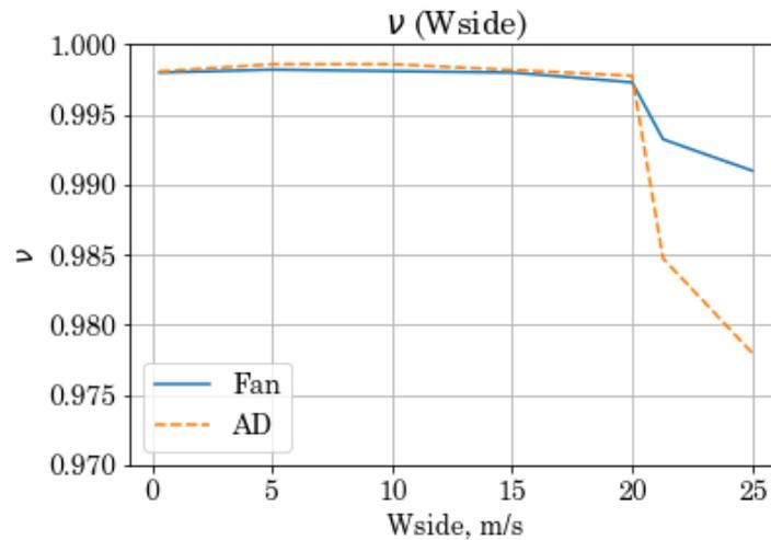
Figure 5: Pressure recovery coefficient by crosswind velocity with the direct **fan** simulation and in the simplified setting – with boundary condition “actuator disk” (**AD**).  $q(\lambda_{en})=0.5$ .
