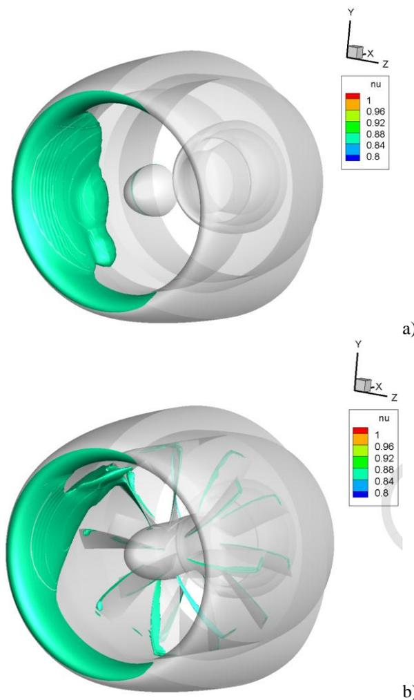
Figure 8: Separation visualization. Iso-surface of coefficient  $\nu = 0.88$  a) with “actuator disk”, b) with fan
