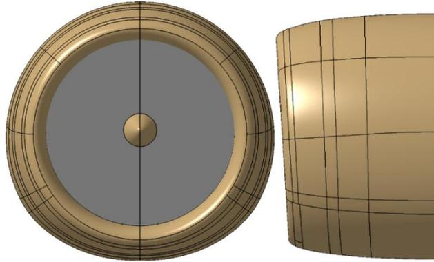
Figure 1: Inlet geometrical model
