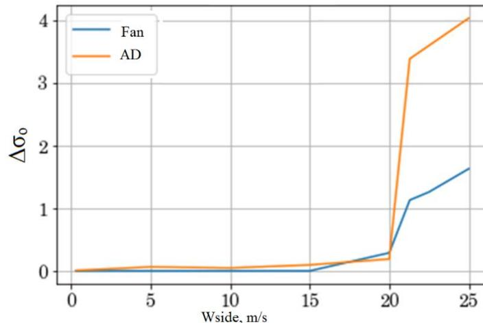
Figure 6: Distortion parameter by crosswind velocity with the direct **fan** simulation and in the simplified setting – with boundary condition “actuator disk” (**AD**).  $q(\lambda_{en})=0.5$ .
