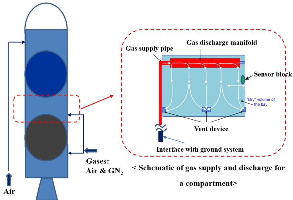
Figure 3: Detailed schematic of thermal control and fire safety system for the inter-tank compartment of test launch vehicle of KSLV-II
