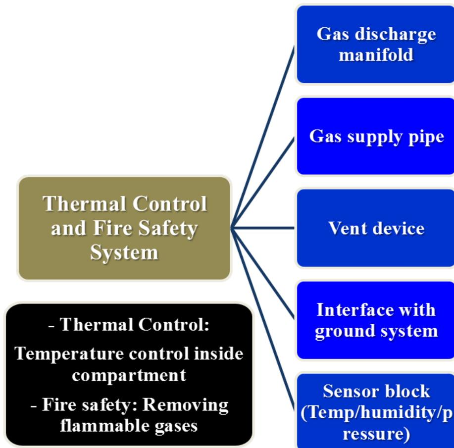
Figure 1: Composition of thermal control and fire safety system for test launch vehicle of KSLV-II
