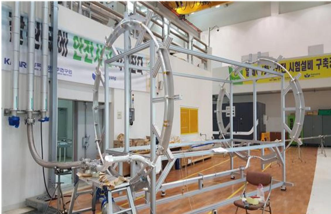
Figure 4: Integration of thermal control and fire safety system of test launch vehicle of KSLV-II
