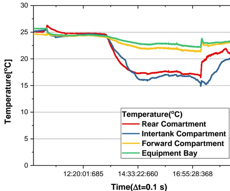
Figure 8: Temperature variation inside the compartments of test launch vehicle of KSLV-II by operation of thermal control and fire safety system during the final stage qualification test
