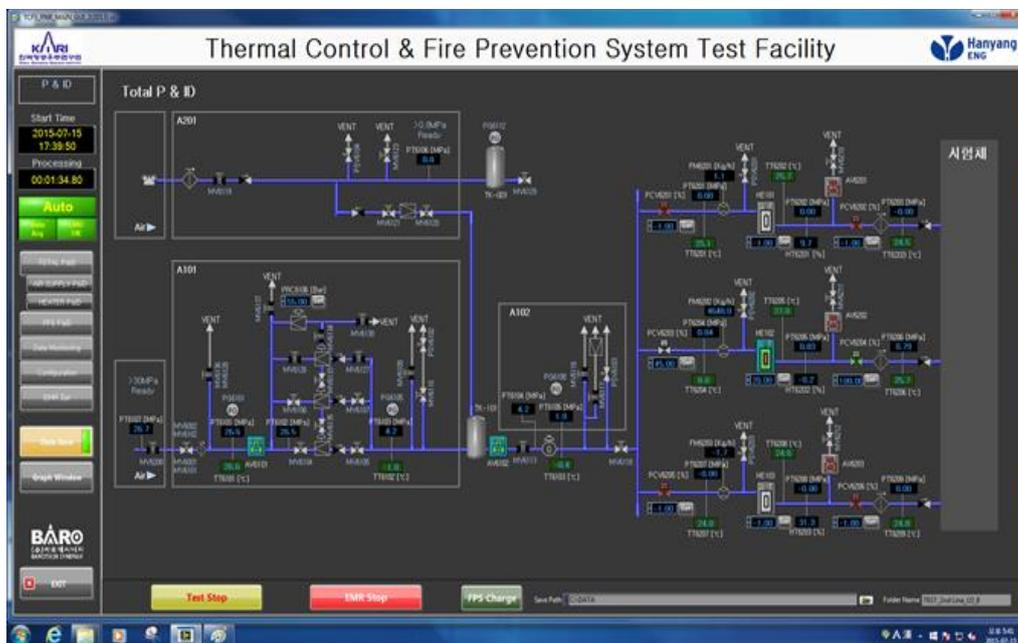
Figure 5: GUI of Thermal Control and Fire Safety Test Facility for Flow Test for TC/FSS
