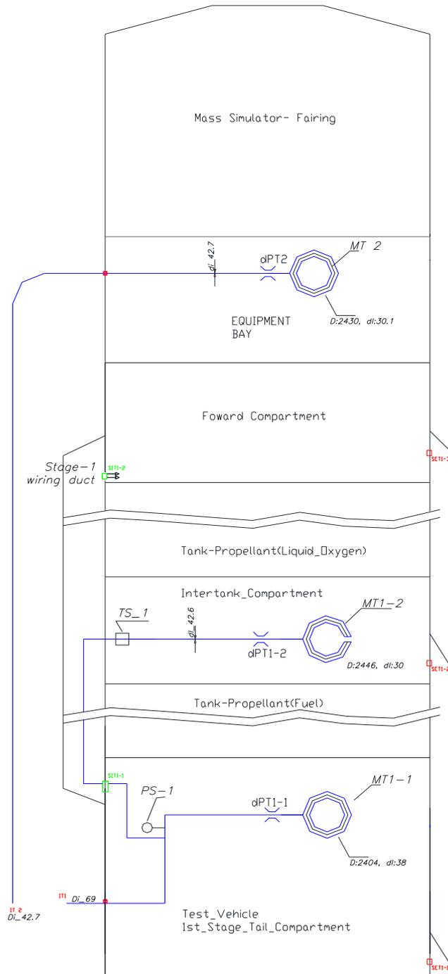
Figure 2: Overall schematic of thermal control and fire safety system for test launch vehicle of KSLV-II
