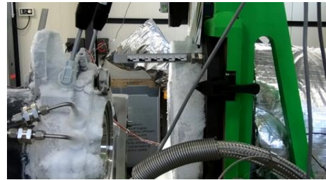
Figure 16: MANG disconnection test
