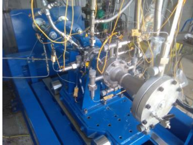
Figure 12: Injector head configured for nitrogen cold flow tests.
