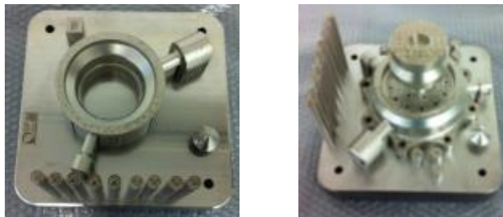
Figure 10: Manufacturing of the injector head components.
