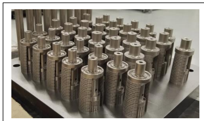
Figure 3: Manufacturing of the injectors after ALM process
