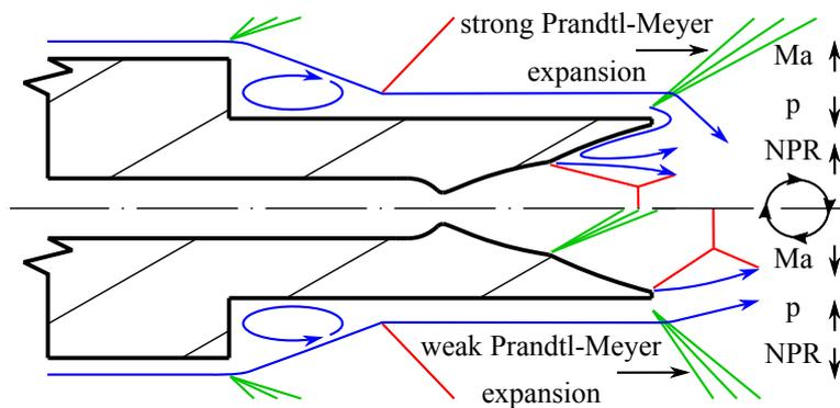
Figure 6: Sketch of the driving mechanism of the flip-flop effect at supersonic external conditions
