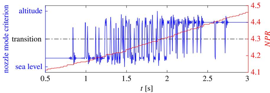
Figure 4: Time vs. nozzle mode criterion at  $Ma_\infty = 1.60$ . Originally published in Bolgar et al. 2019<sup>4</sup>.
