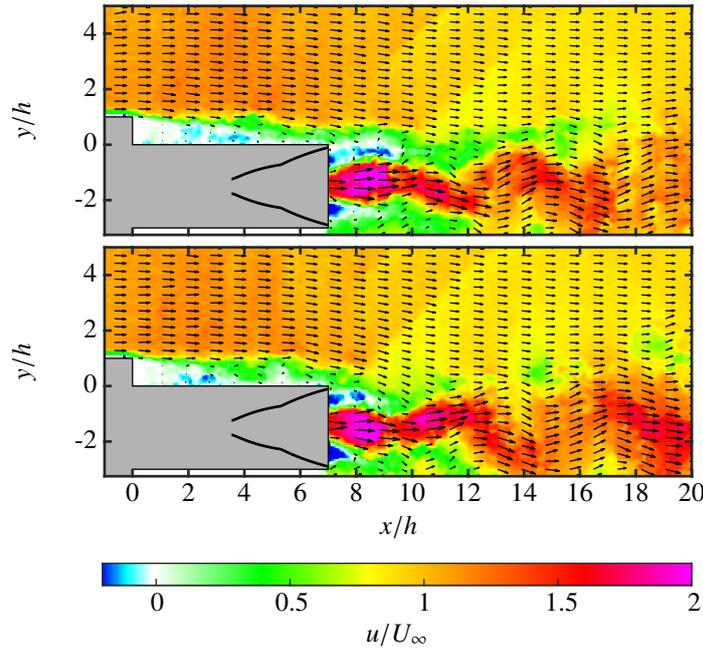
Figure 7: Illustration of the streamwise component of instantaneous vector fields at  $Ma_\infty = 0.80$  with  $NPR = 7$ . Refer to Bolgar et al.<sup>4</sup> for more details on the measurements.
