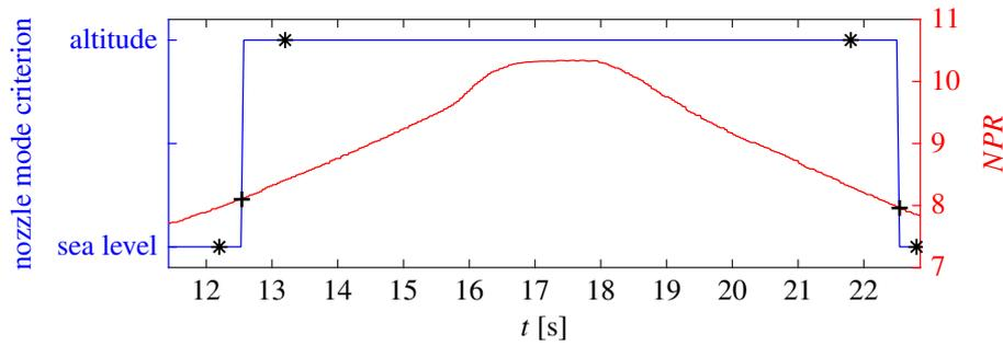
Figure 3: Time vs. nozzle mode criterion at  $Ma_\infty = 0.80$ . Asterisks provide the instance of the schlieren images provided in figure 5. The + signs indicate the moment of transition and retransition.
