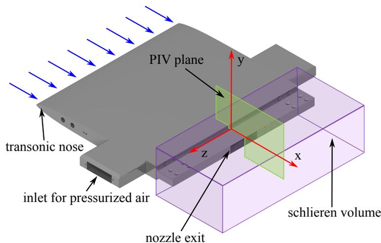
Figure 2: Illustration of the planar space launcher model with a 2D Dual-Bell nozzle and the measurement locations for PIV and schlieren
