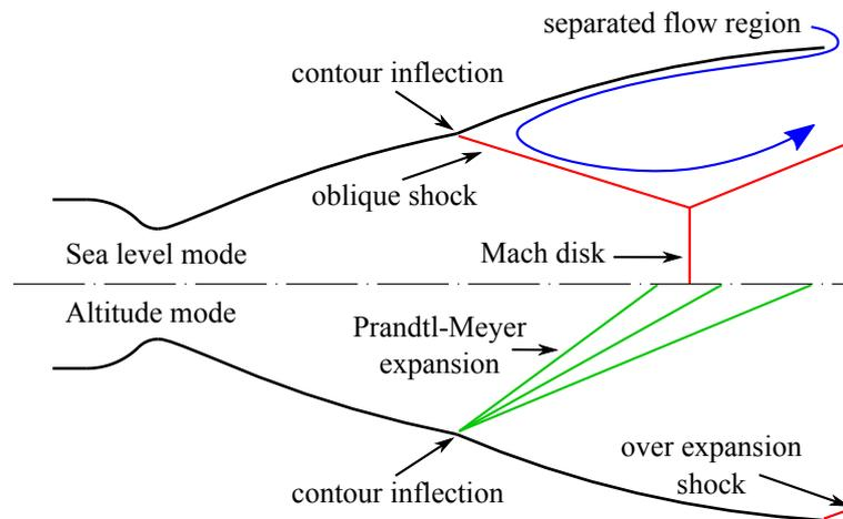
Figure 1: 2D sketch of the two Dual-Bell operating modes: Sea level mode is illustrated above the axis of symmetry. Altitude mode is illustrated below the axis of symmetry.
