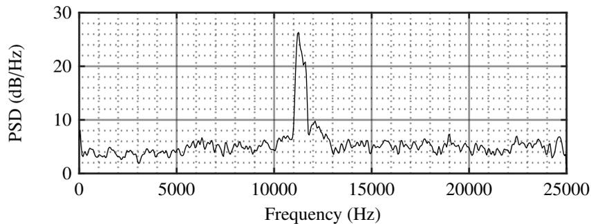
Figure 10: Frequency vs. PSD of the light intensity in the schlieren recordings in figure 9
