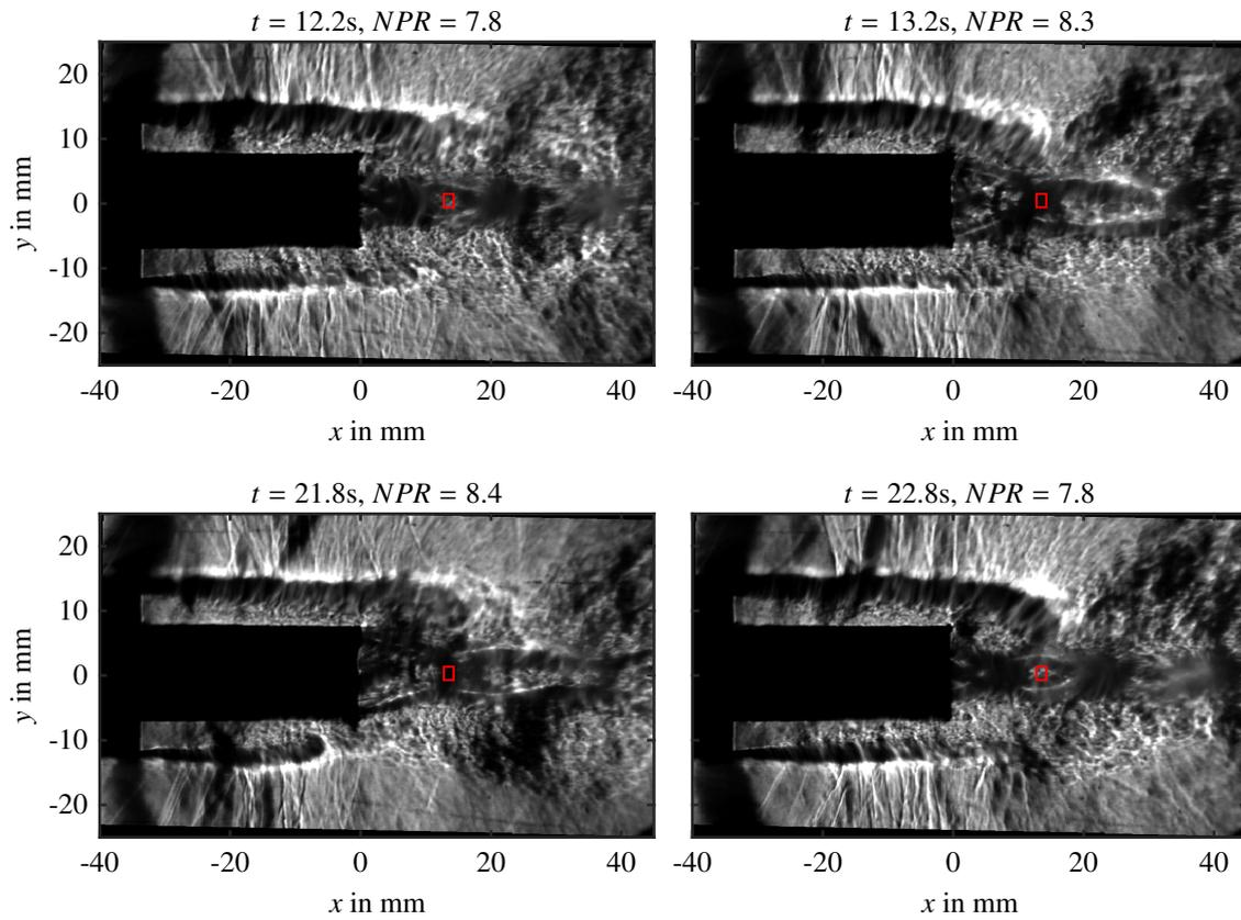
Figure 5: Schlieren recordings of the nozzle transitioning and retransitioning with increasing and decreasing  $NPR$ , respectively. The red box in the images illustrates the interrogation window for the nozzle mode criterion.
