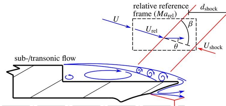
Figure 8: Graphical illustration of the calculation method of the screech frequency
