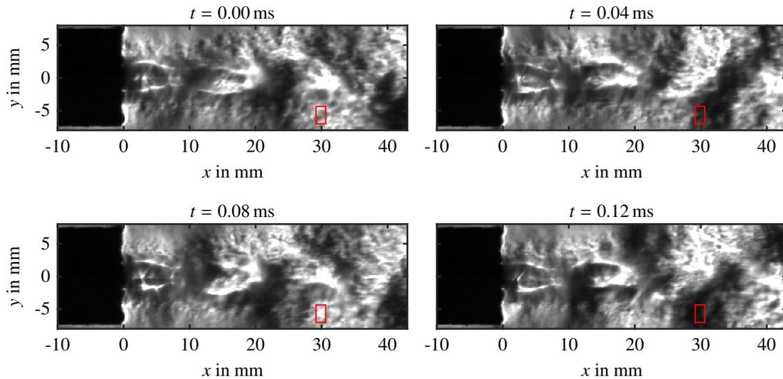
Figure 9: Schlieren recordings of the nozzle in sea level mode. The alternating bright and dark patches indicate coherent changes in the density gradient. The red box in the images illustrates the interrogation window for the FFT.
