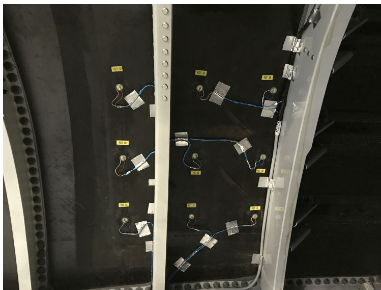
Figure 5: GRA instrumented skin section.
