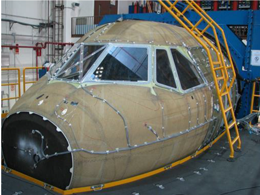
Figure 4: Green regional aircraft demonstrator cockpit
