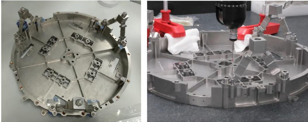
Figure 10: Bipods mounting(a), CMM Measurements (b)
