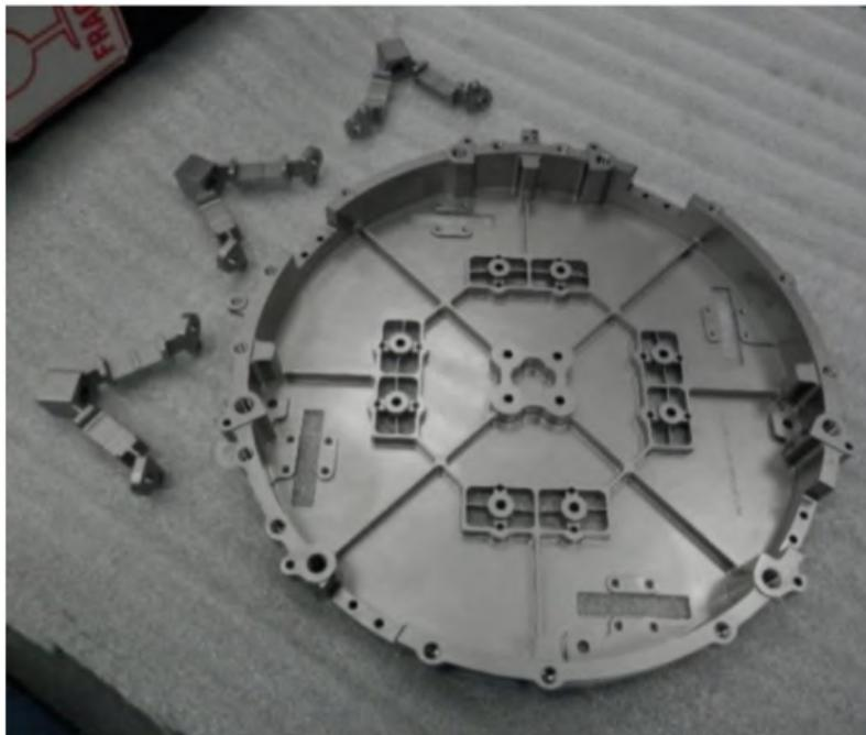
Figure 4: FPA Support Structure and Bipods
