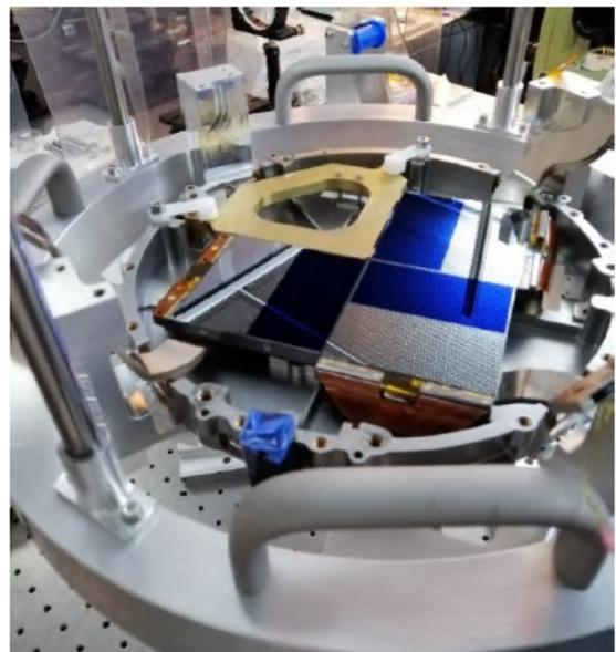
Figure 12: CCDs mounting in FPA
