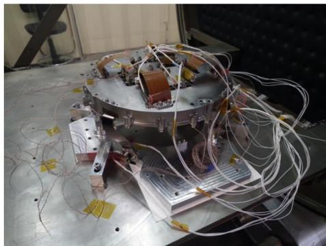
Figure 14: PLATO FPA Prototype inside the chamber
