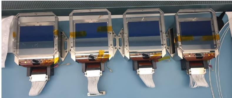
Figure 8: PT-100 Mounting on CCDs
