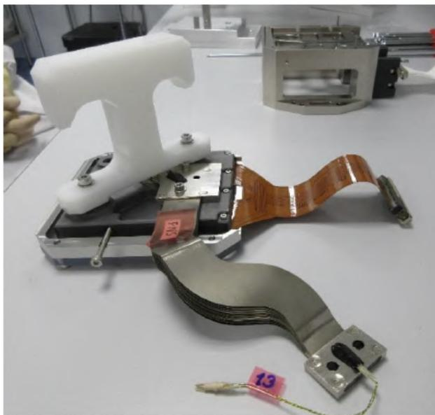
Figure 11: Thermal straps in CCDs.
