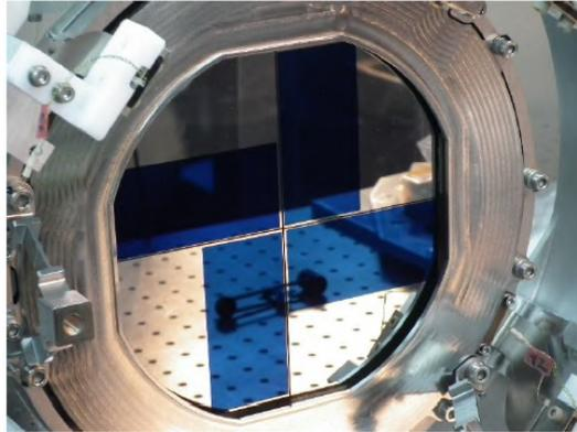
Figure 13: FPA with Straylight Mask and Bipods
