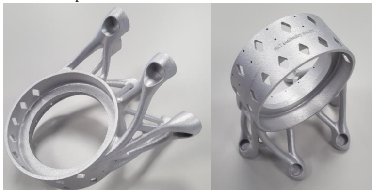
Figure 15: Scalmalloy® demonstrator after finishing operations
