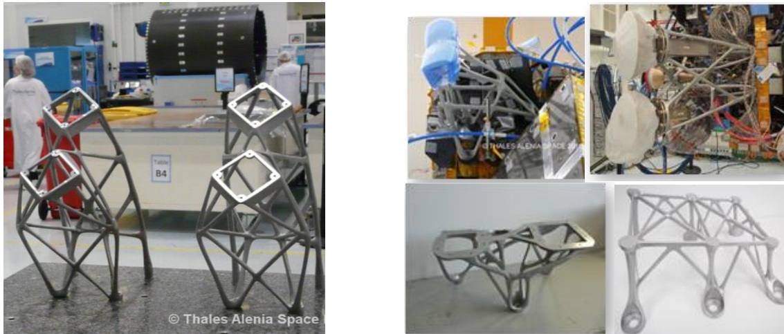
Figure 1: Examples of THALES ALENIA SPACE aluminum LBM secondary structures flight models. From left to right: TTC Antenna support and Ku Horn support of Koreasat 5A and Koreasat 7 (in orbit since May 2017), Antenna support and Ku horn support of Inmarsat Hellasat 3 (in orbit since June 2017), TMTC support of Telkom 3S (in orbit since February 2017) and the Banghabandu shimplate (in orbit since 2017)
