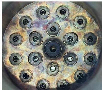
Figure 19: Firing-Plate after test campaign completion
