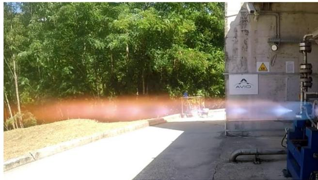
Figure 6: FSBB firing-test. Test06 (48.51 bar)
