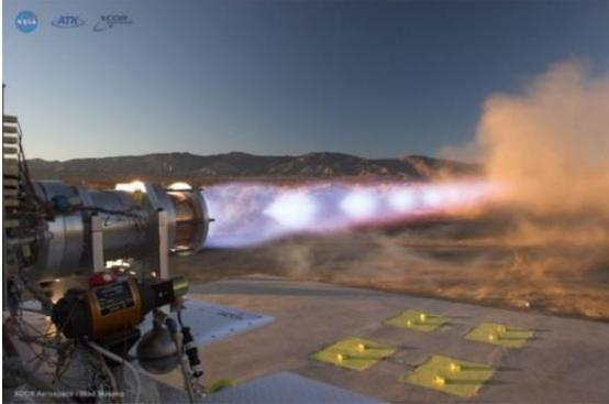
Figure 1: XCOR test firing of a 33kN LOX/methane engine
