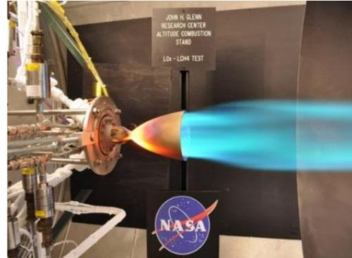
Figure 2: Aerojet 100-lbf LOX/LCH4 reaction control engine in test at NASA GRC
