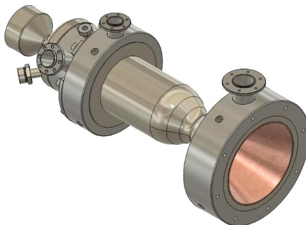
Figure 3: Sketch view of HYPROB DEMO test-article.
