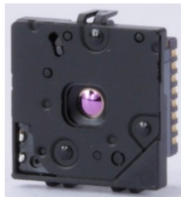
Figure 10: FLIR Lepton 3.5 infrared camera
