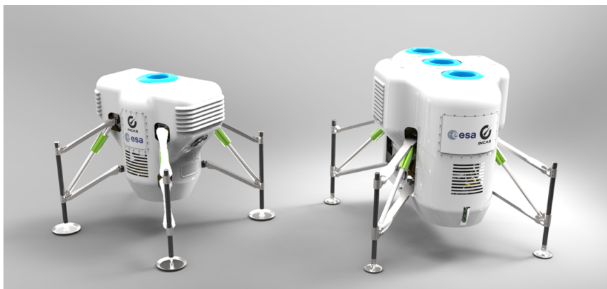
Figure 1: The DTV vehicle: 61.6 [Kg] single engine or 126.62 [Kg] triple engine configuration, 1.2 [m] total height. Courtesy of INCAS.
