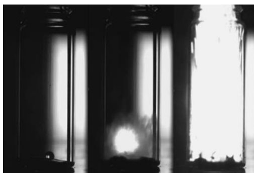
Figure 8: Hypergolic reaction of TMEDA gel with hydrogen peroxide (sequence from high speed video recording).
