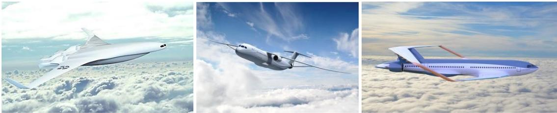
Figure 1: Concepts for Blended Wing Body from “Silent Aircraft Initiative”, Truss Braced Wings from “SUGAR” project and Box-Wing from “PARSIFAL” project
