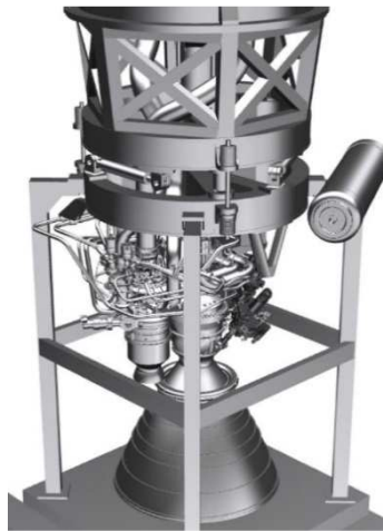
Figure 16: Handling stand for PROMETHEUS engine installation at P5 (Courtesy of DLR)
