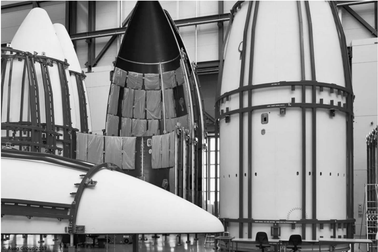
Figure 1: Payload fairings at RUAG Space, where the FAP mats used today are shown [2].
