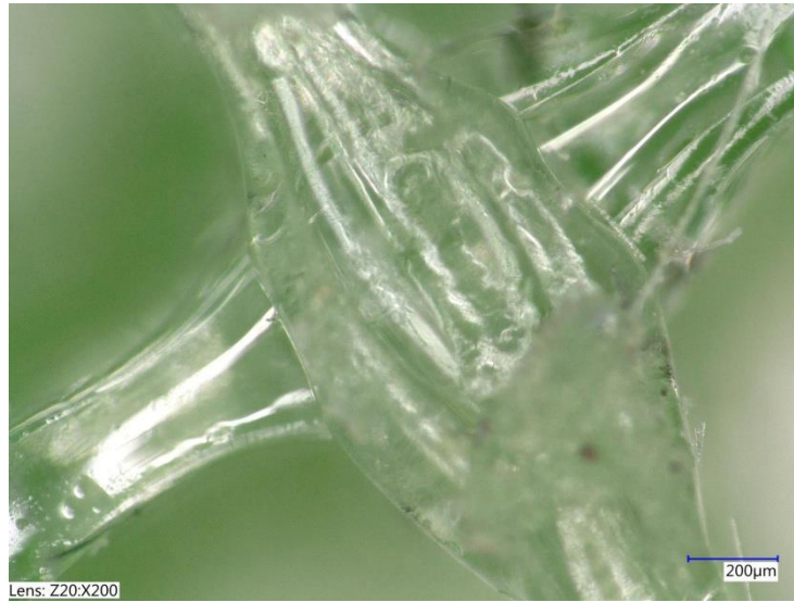
Figure 4: Infill covered be resin.
