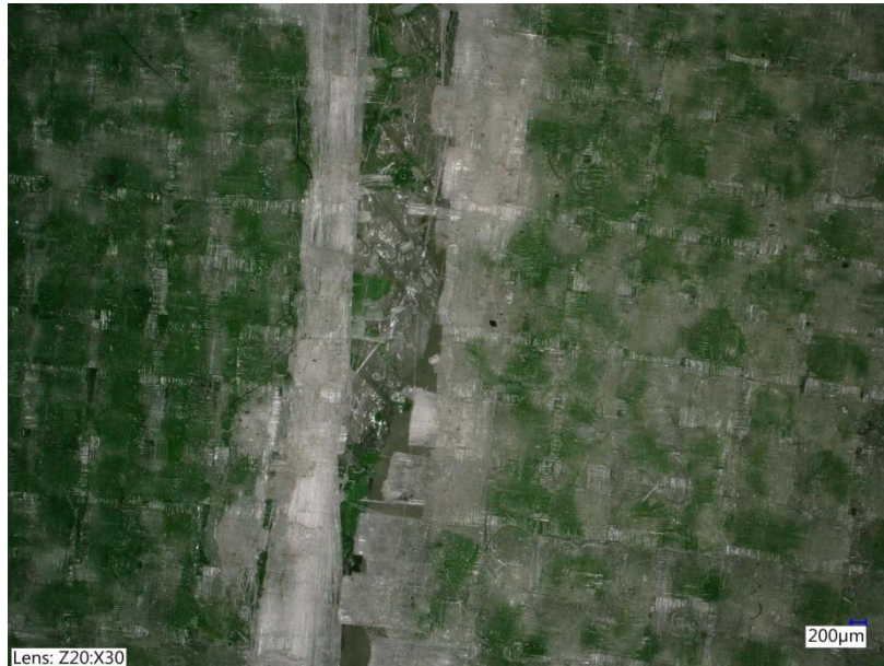
Figure 14: Destroyed sample with 100% infill.
