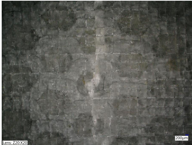
Figure 13: Stress propagation inside honeycomb core composite
