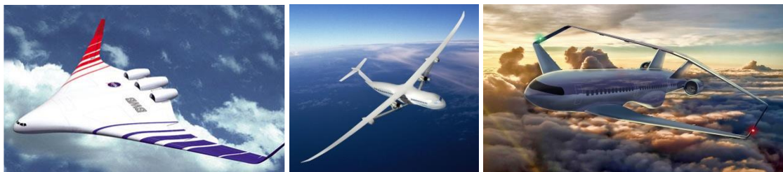
Figure 1: Blended Wing Body (BWB), Truss Braced Wings (TBW) and PrandtlPlane (PrP) concepts
