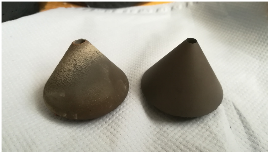
Figure 9: Comparison between tip status: left post-firing (left) and pre-firing (right)
