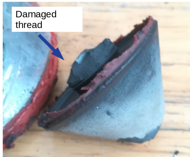
Figure 8: Tip suffering from thread failure
