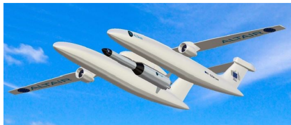
Figure 6: View of the carrier with the launcher attached
