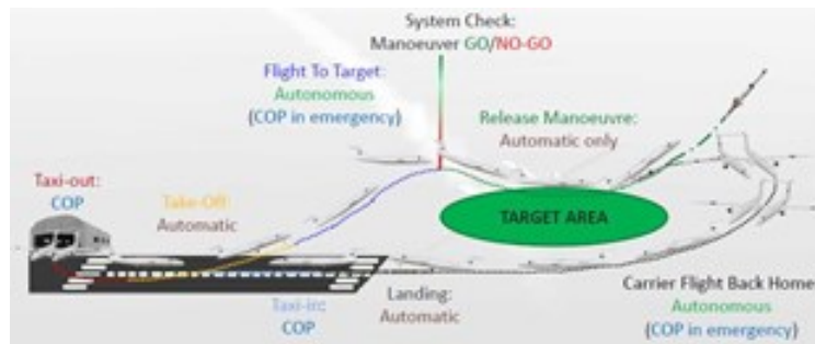
Figure 5: ALTAIR CONOPS: COP (Carrier Operator) vs. Autonomous Operation
