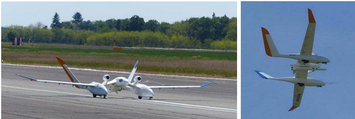
Figure 20: EOLE equipped with the ALTAIR experimental systems during the May 2019 Saint-Yan flight tests
