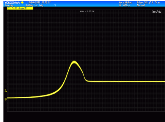
B) SSPC with soft start (Current under 15 A)
