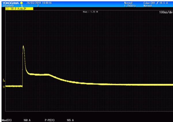
A) Electromechanic Contactor (Current over 150 A)
