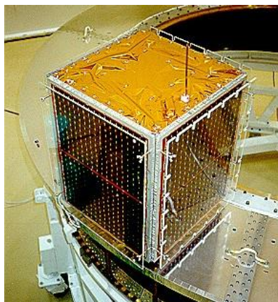
Figure 1: UPM-Sat 1 assembled in the adapter platform ASAP of the Ariane IV-40 launcher.
