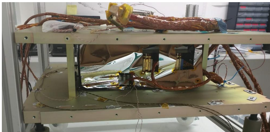
Figure 4: Battery mounted on the spacecraft and wrapped in SLI.
