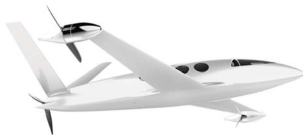
Figure 12: Model of the all-electric airplane ALICE [13]
