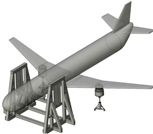
Figure 5: Aircraft suspending on combined ESS
