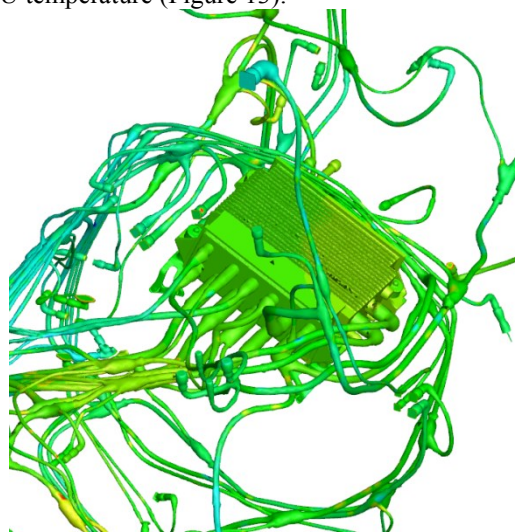
Figure 11. Baseline Configuration : ECU Temperature map
