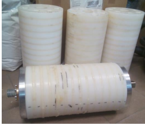
Figure 3 - Multiport HDPE Fuel grains manufactured in IoA.
