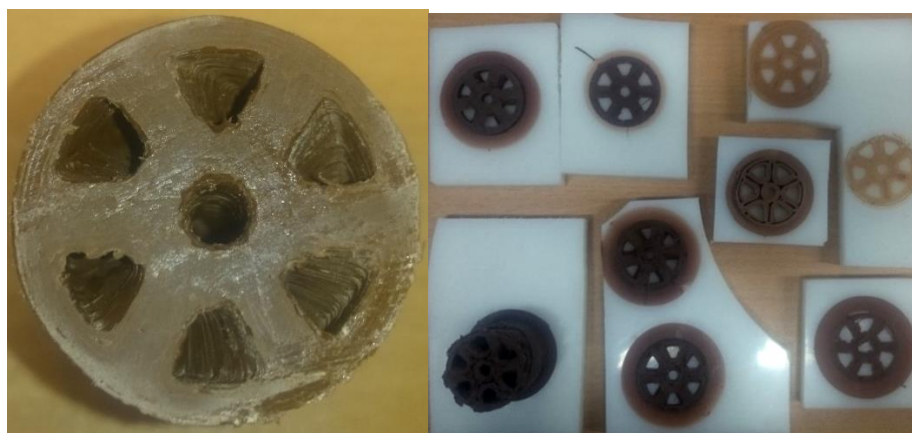
Figure 5 -Failed attempts of HDPE grains
