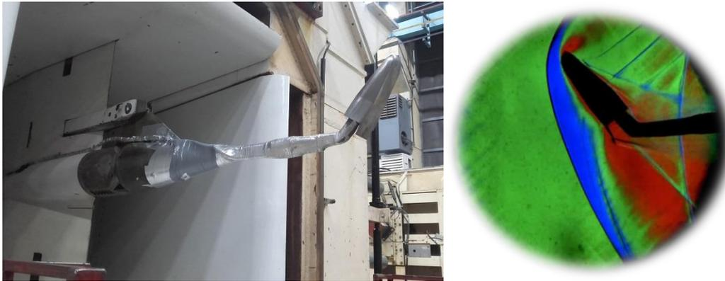
**Figure 1: Space Rider WTT at INCAS trisonic facility - Mach = 1.4 AoA = 60 deg**
