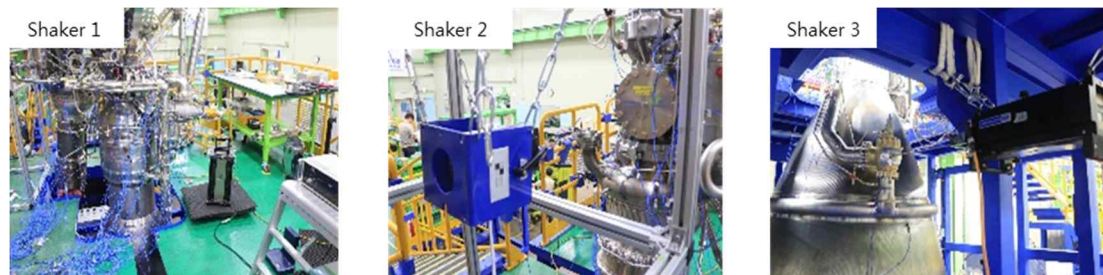
Figure 7: Excitation setup using the electro-dynamic shaker
