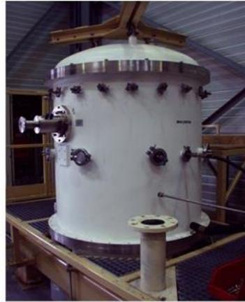
Brake test in vacuum chamber
