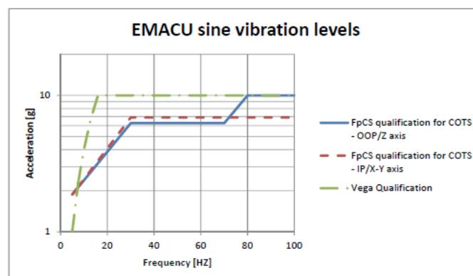
Figure 14 : Sine vibration requirement for IXV EMACU
