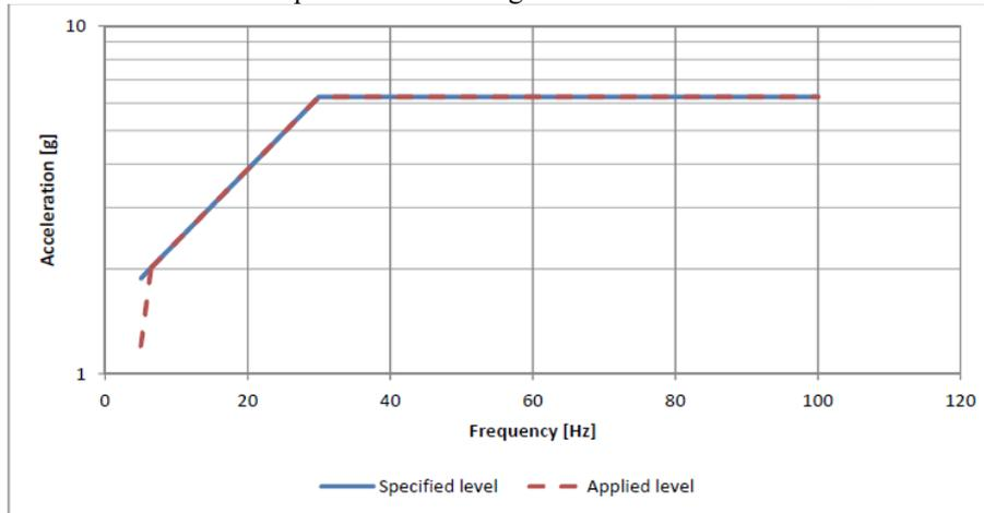
Figure 11 : Sine vibration requirement for IXV EMA
