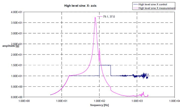
Figure 16 : Sine vibration results for EMACU
