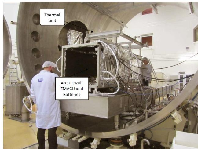
Figure 6: Thermal tent in vacuum chamber at the Centre Spatial de Liège (Belgium).
