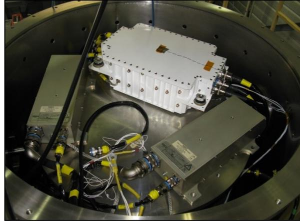
Figure 10 : FpCS Electronics and Batteries inside vacuum chamber
