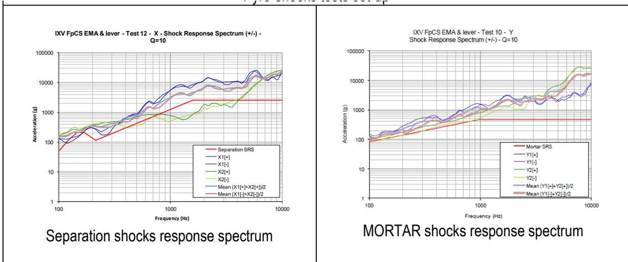
Figure 6: Pyro-shock tests
