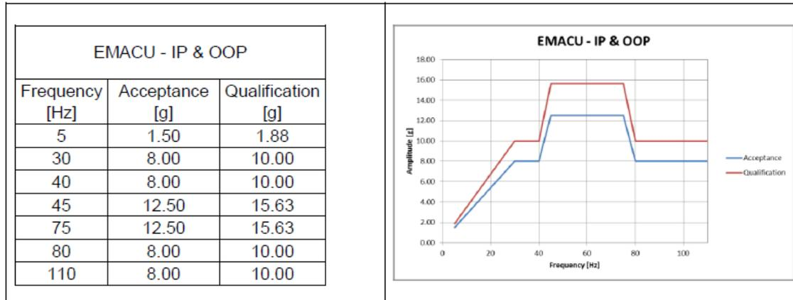
Figure 15 : Sine vibration requirement for SR EMACU
