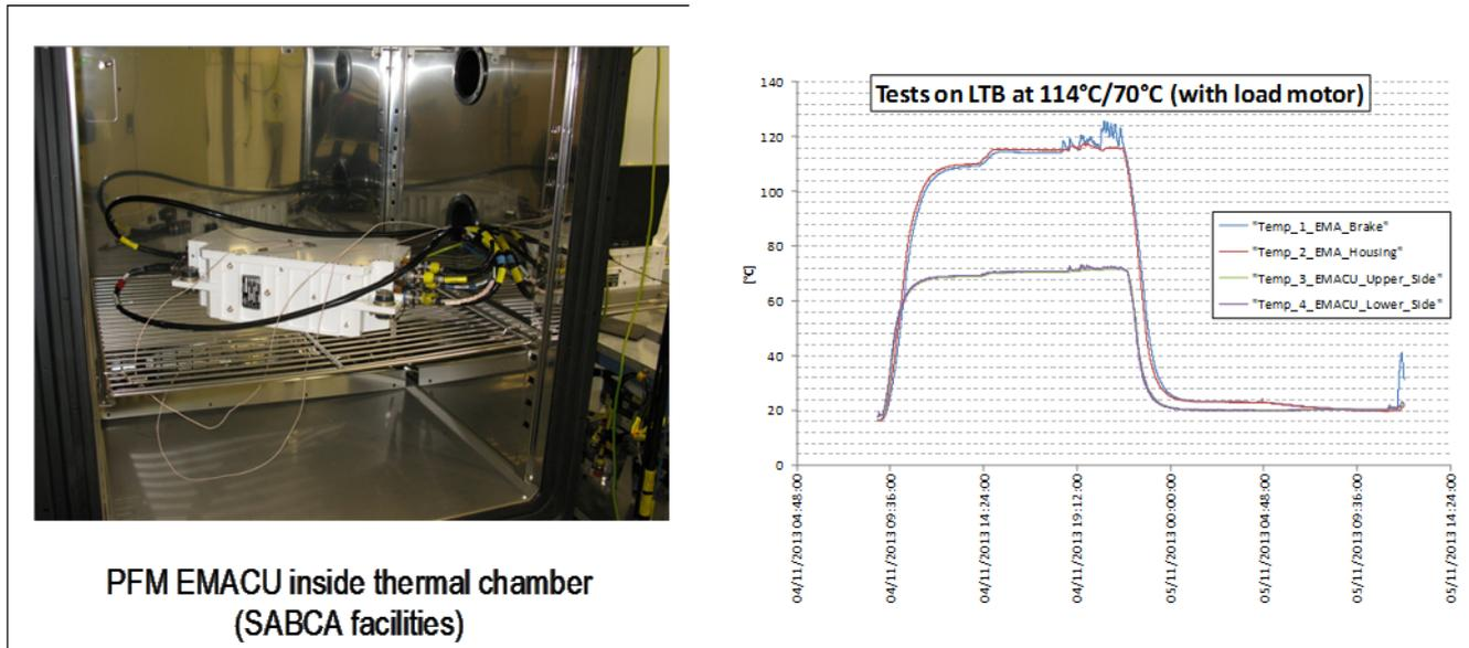
Figure 10 : PFM EMA & lever, EMACU - Temperature tests under external load
