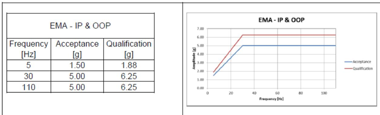
Figure 12 : Sine vibration requirement for SR EMA
