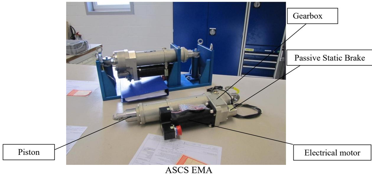
This heritage contains also the brake system, added w.r.t. VEGA design in order to block the flap control system during its inoperative phase. The qualification perform in the frame of IXV program is partially reuse to justify requirements which have not changed.
