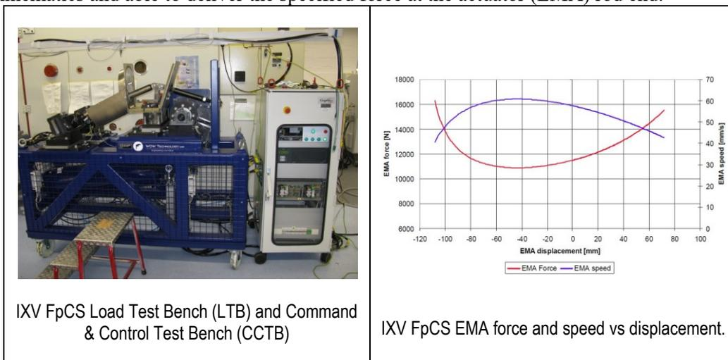
Figure 8 : Mechanical tests on EMA and lever
