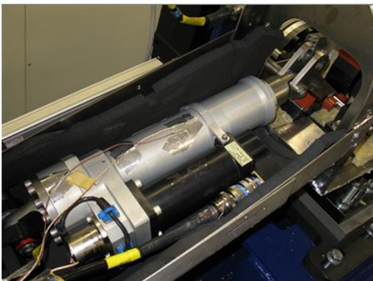
PFM EMA (S003) and lever (S003) in thermal enclosure on Load Test Bench (LTB).
